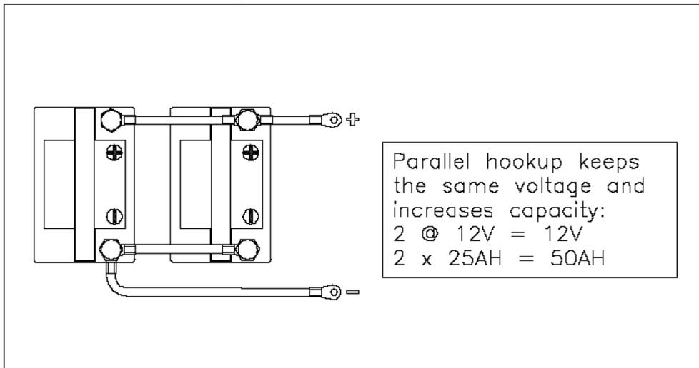
Figure 5-2. Parallel Connection
