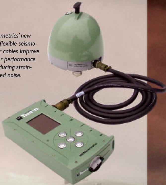
The highly successful Trillium 120 is now available with motorized mass centering. This new version maintains exceptional performance over a wide temperature range with the added benefit of fast "one-touch" mass centering. Motorized mass centering simplifies seismometer installation and gives customers the option of remotely re-centering the masses via a telemetry connection.
