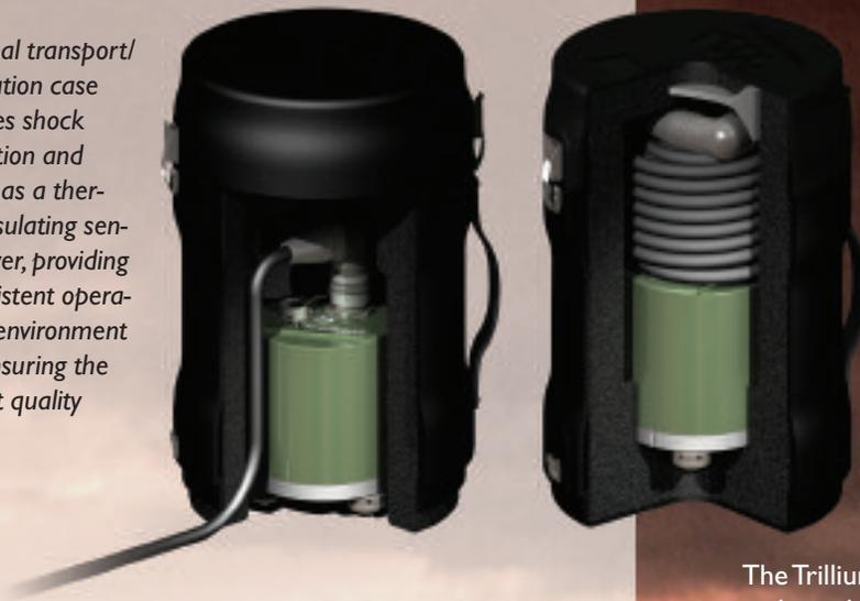
Trillium Compact combines the superior performance of a broadband seismometer with the installation convenience of a rugged geophone. The instrument incorporates a symmetric triaxial force feedback sensor design with a response flat to velocity from 120 seconds to 100 Hz.
