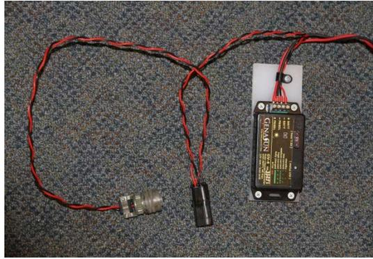
**Genasun GV-4 charge controller, wired internally to 4 pin bulkhead**
