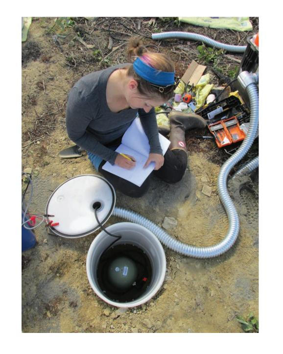
Figure 9. In July 2013, Tim Parker and Kasey Aderhold (pictured), a PASSCAL student intern, installed two Trillium 120PA sensors in PASSCAL temporary vaults.
