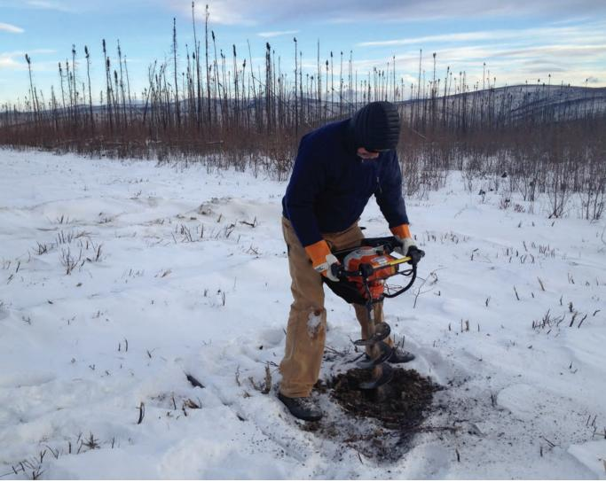
Figure 6. Tim Parker augering the first of 3 holes for directly buried sensors. Sensors are emplaced in loess resting on weathered schist bedrock. Holes are 20 cm in diameter, separated by 1.3 m.
