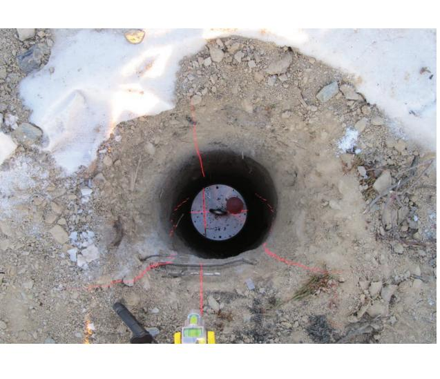
Figure 8. Orienting the T120PHQ. A North line is machined into the top plate of the sensor and illuminated with a laser to translate the compass north line to sensor.
