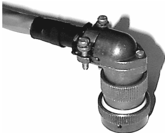
Figure 44: Completed assembly of EpiSensor end of cable 840356
