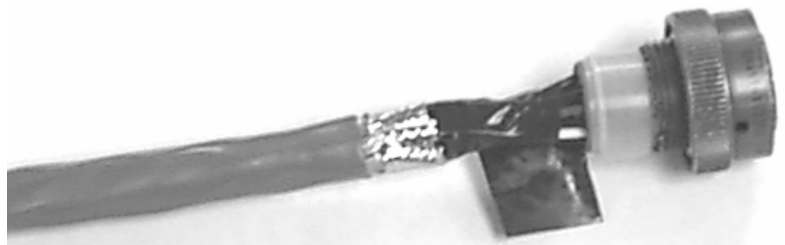
Figure 32: Wrapping the connection with PVC tape
