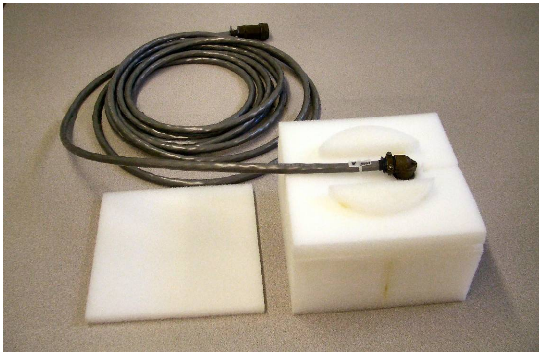
Figure 7: Second Packaging Piece Installed over Connector Shell
