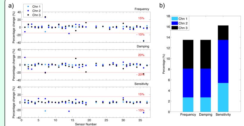
Figure 5. a) Percentage change between frequency, damping, and sensitivity values before and after the experiment, for each sensor, for each channel. b) Percentage of channels which present a change greater than 15% for frequency and sensitivity, and 20% for damping.
