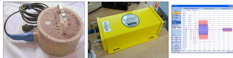
Figure 1. Sercel L-22 sensor (left), DAQLink-II unit and example of Bird Dog test (right).
