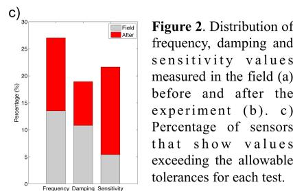
Figure 2. Distribution of frequency, damping and sensitivity values measured in the field (a) before and after the experiment (b). c) Percentage of sensors that show values exceeding the allowable tolerances for each test.
