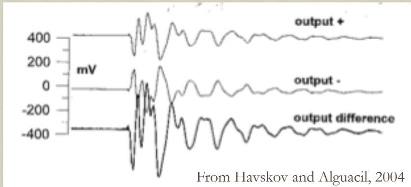
If the noise (right) were to be induced in the sensor cable, it should be similar on both output wires. Taking the difference of the output traces subtracts out the noise, but adds the signal.
