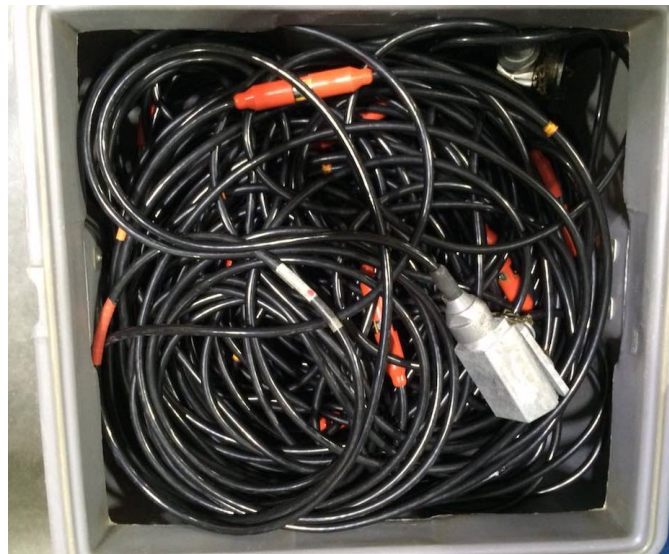
Figure 7. Proper Spaghetti-style method for storing Geode cables
