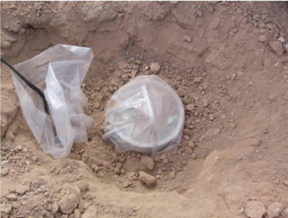
Pack dirt or sand along the outside of the bag all the way up the sensor and gently compact to keep the sensor level.
