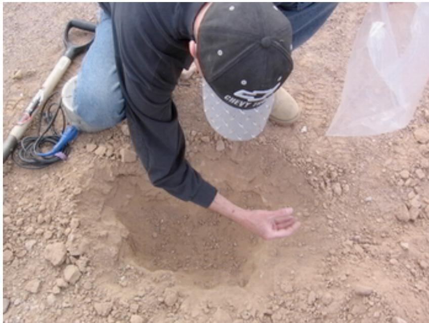
**Tip 4** – For a short-term experiment (less than 2 months, and not very wet environment) direct burial of the L-22 is okay. For a long-term experiment (more than 2 months) or in a very wet environment the sensor should be protected from flooding by burying it in a plastic bag. Place the instrument in the bag with the top of the bag open in your pit.
