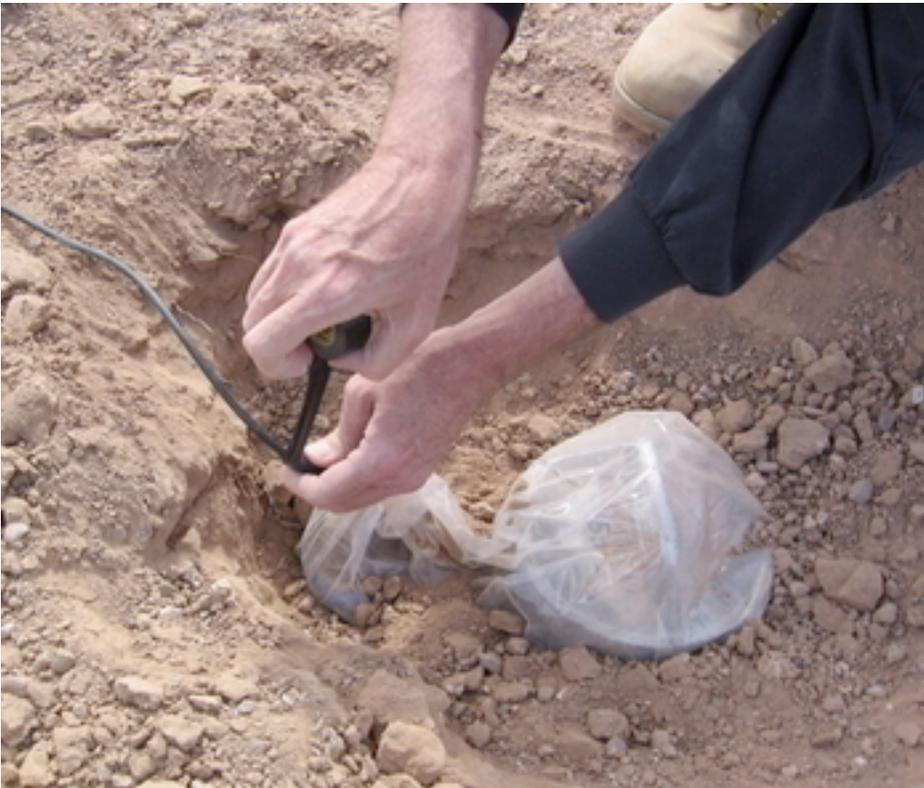
Check the orientation and bubble level one last time, then close the bag and secure with electrical/waterproof tape. Evacuate any air remaining in the bag.
