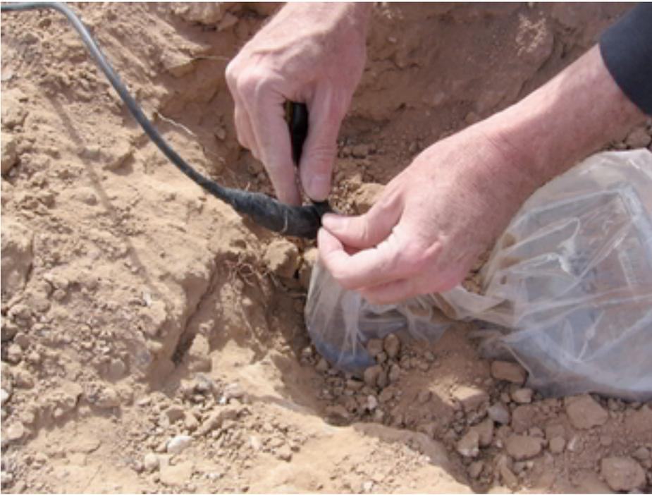
Tape around the cable just beyond the connection into the sensor and seal all open edges of the bag.
