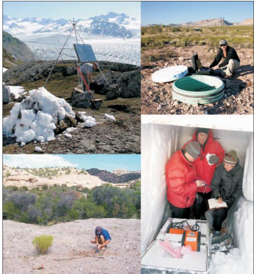
Fig. 2. Recent representative PASSCAL projects in the field. Clockwise from upper left: Columbia Glacier passive seismic recording (Dan McNamara, U.S. Geological Survey); EarthScope USArray Transportable Array station Y22C at New Mexico Institute of Mining and Technology near Socorro, New Mexico (Marcos Alvarez, IRIS Consortium); SOUTHBERG seismic vault on iceberg C16, McMurdo Sound, Antarctica (Doug MacAyeal, University of Chicago); Arizona Source Phenomenology Experiment, active source recorder deployment (Travis Glen, Southern Methodist University and Bill Walter, Lawrence Livermore National Laboratory, U.S. Department of Energy).
